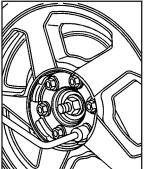
2. Turn the wheel wrench counterclockwise to loosen the wheel nuts. Do not remove them yet. If your vehicle has locking lug nuts, the key is supplied in the tool bag. Use the key along with the wheel wrench to remove the wheel nuts from the tire.
